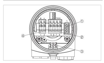
Electronics and terminal compartment, single chamber housing
