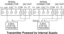
Fransmitter Powered by Internal Supply (optional)
