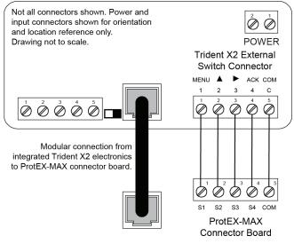
Integrated Trident X2 (PD8-765) Required Connections
