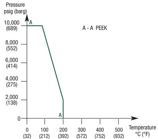
**Standard product specification:** supplied in 316 stainless steel with PEEK soft seat, PTFE packed, T bar operation, 10,000 psig (689 barg) maximum pressure rating, 200C maximum temperature rating.
