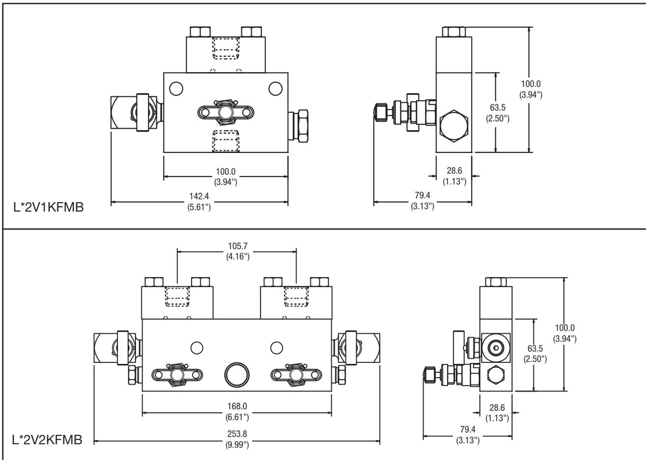
Overall width with valves fully open
