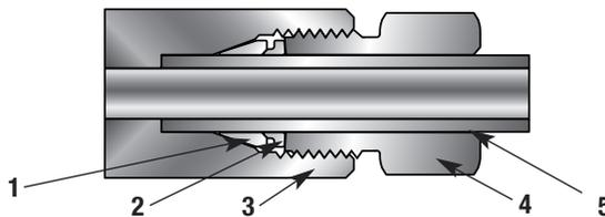
1. Front ferrule with corrosion-resistant Parker SUPARCASE® forms a tight pressure seal between the body and ferrule in a *second* strong mechanical hold on the tube.
