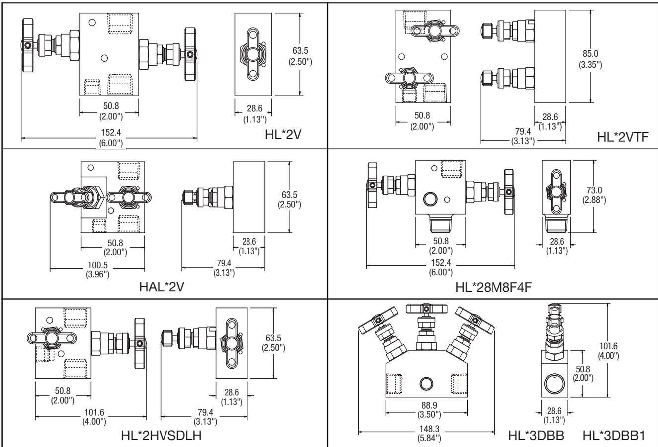
\*Overall width with valves fully open
