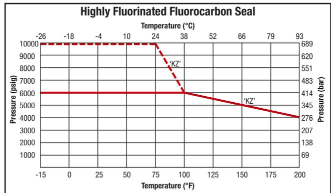
Note: To determine MPa, multiply bar by 0.1 Key: — 6,000 psi - - - 10,000 psi
