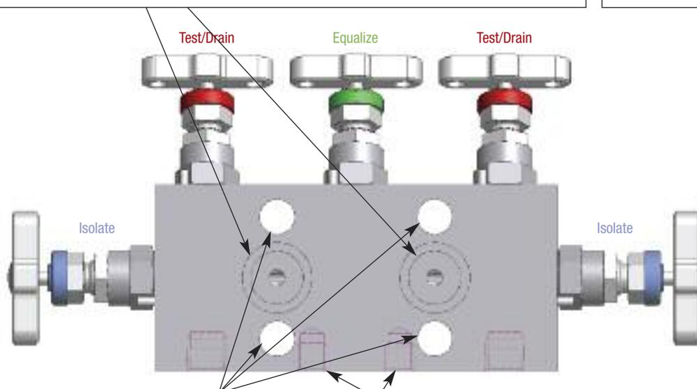
**Manifold to transmitter mounting:** all direct mount manifolds are provided with 4 off 7/16 UNF x 1.625" high tensile zinc plated carbon steel bolts. Bolt holes are standard on 54mm/2.125" centres. Optional St. bolts are available.
