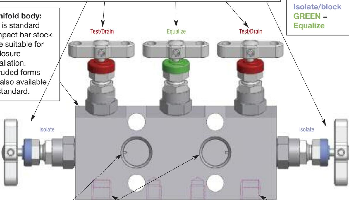
**Process inlet connections** positioned on front face 1/2" NPT female threads or kidney flange/oval/futbol are standard. Alternative thread forms, socket or butt weld and PTFree connections are available. Standard connections are on 2.125"/54mm.
