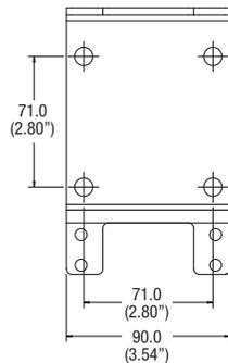
Simple to install bracket on horizontal or vertical 2" standpipe. Designed for horizontal or vertical mounting of manifold giving total installation flexibility.
