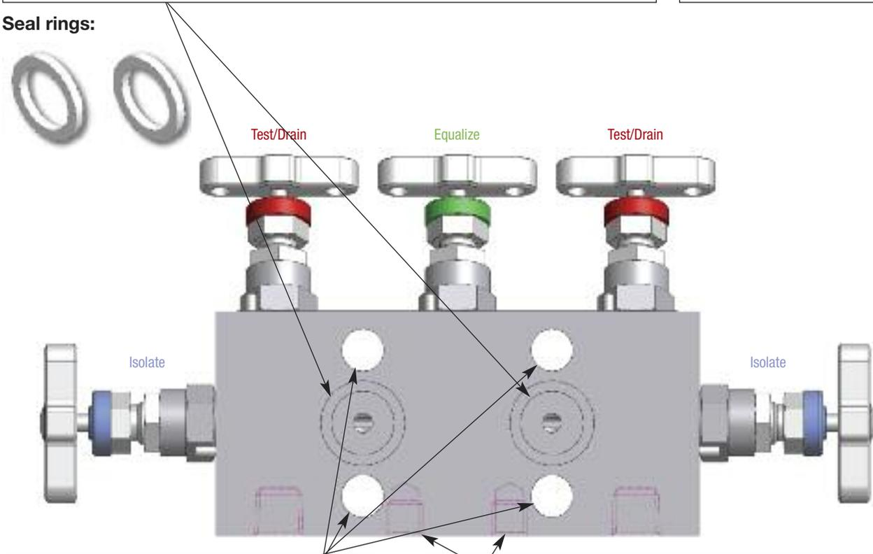
**Manifold to transmitter mounting:** all direct mount manifolds are provided with 4 off 7/16 UNF x 1.625" high tensile zinc plated carbon steel bolts. Bolt holes are standard on 54mm/2.125" centres. Optional St. St. bolts are available.
