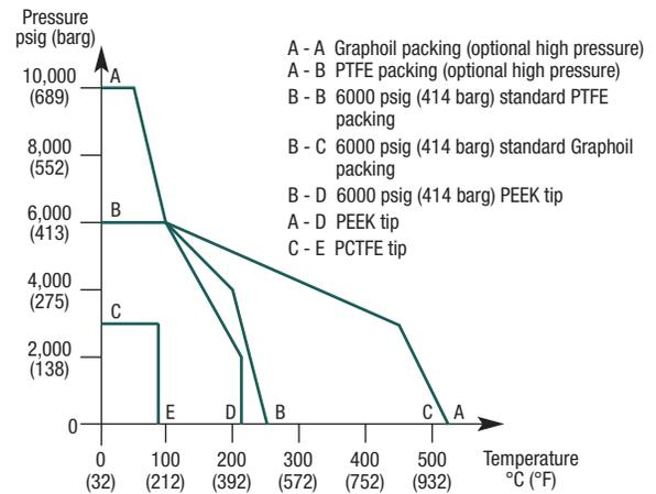
**Standard product specification:** metal/metal seated, PTFE packed, stainless steel, T bar operation, globe pattern, 6000 psig (414 barg).
