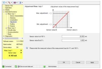
Fig. 13: Example of a DTM view - Adjustment
