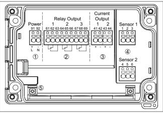
Fig. 6: Wiring plan VEGAMET 842
