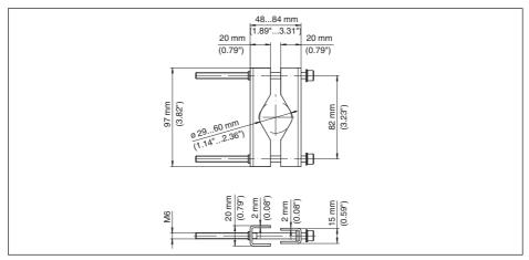
Fig. 27: Dimensions Brackets for tube mounting
