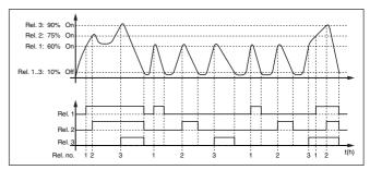
Fig. 19: Example of pump control 4
