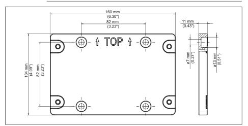
Fig. 25: Dimensions mounting plate
