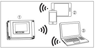
Fig. 2: Wireless connection to standard adjustment tools with integrated Bluetooth LE or alternatively Bluetooth USB adapter.
