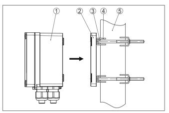
Fig. 4: Tube mounting
