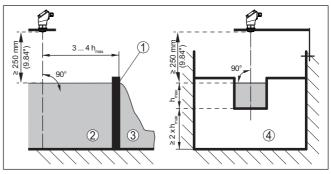
Fig. 22: Flow measurement with rectangular flume:  $\mathbf{h}_{\max} = \max.$  filling of the rectangular flume
