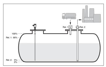
Fig. 14: Example of level measurement, horizontal cylindrical tank
