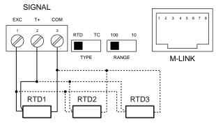
Figure 8. Average Temperature RTD Input Connections
