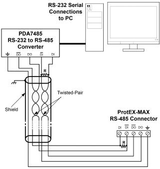
Figure 11: RS-485 Wiring
