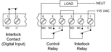
**Figure 18. Interlock Connections**
