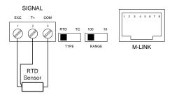
Figure 5. Three-Wire RTD Input Connections
