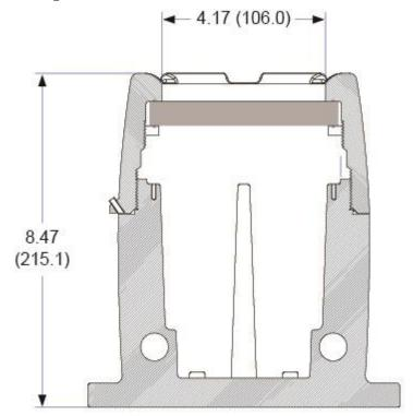
Figure 24: Enclosure Dimensions - Side Cross Section View
