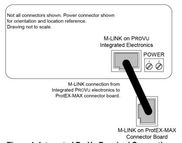
Figure 1: Integrated ProVu Required Connections
