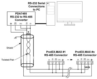
Figure 12: RS-485 Two-Wire Multi-Drop Wiring
