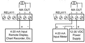
Figure 17. 4-20 mA Output Connections
