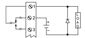
Use a diode with a reverse breakdown voltage two to three times the circuit voltage and forward current at least as large as the load current.
