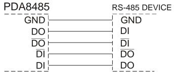
Figure 21: General Four-Wire Network Connection
