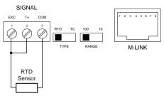
Figure 6. Two-Wire RTD Input Connections
