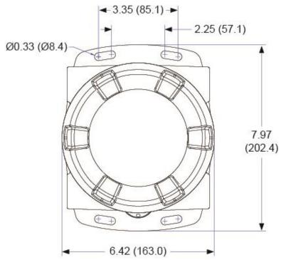
Figure 23: Enclosure Dimensions – Front View
