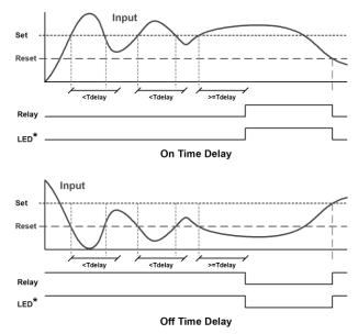
When the signal crosses the set point, the *On* time delay timer starts and the relay trips when the time delay has elapsed. If the signal drops below the set point (high alarm) before the time delay has elapsed, the *On* time delay timer resets and the relay does not change state. The same principle applies to the *Off* time delay.
