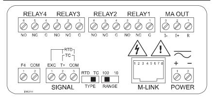
Figure 2. Connector Labeling for Fully Loaded PD8-7000
