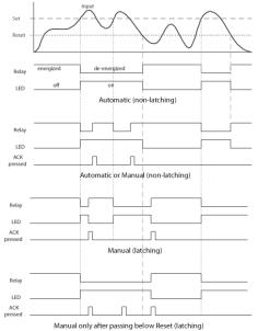
Note: Relay coil is energized in non-alarm condition. In case of power failure, relay will go to alarm state.
