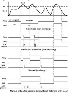
For Manual reset mode, ACK can be pressed anytime to turn "off" relay. To detect a new alarm condition, the signal must go below the set point, and then go above it.
