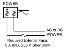
**Figure 3. Power Connections**
