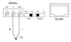
Figure 4. Thermocouple Input Connections
