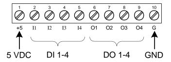
Figure 19: Digital I/O Connections
