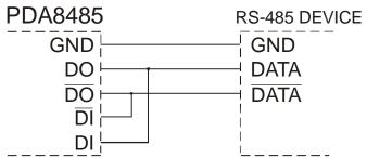
Figure 22: General Two-Wire Network Connection
