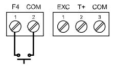
Figure 16. F4 Digital Input Connections
