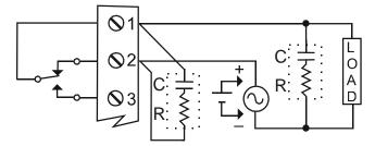
Figure 14. AC and DC Loads Protection
