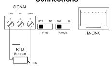
Figure 7. Four-Wire RTD Input Connections
