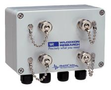
Wilcoxon's cable termination junction boxes are a low cost monitoring solution for 1-4 channel applications. The CB series are NEMA 4X rated for use in harsh environments and come with cap covers to protect against dust and water intrusion. Predrilled inputs allow fast cable installation. Wilcoxon also offers the CBT series for compatibility with triaxial sensors.
