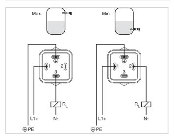
VEGASWING 51 with valve block according to ISO 4400
