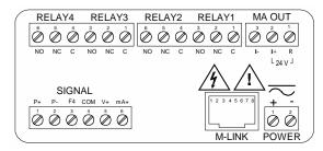
Figure 10. PD6200-##7 Connectors Label
