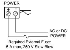
**Figure 11: Power Connections**
