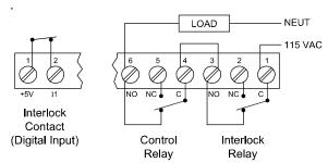
Figure 24. Interlock Connection
