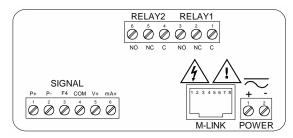
Figure 6. PD6200-##2 Connectors Label
