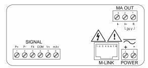
Figure 7. PD6200-##3 Connectors Label
