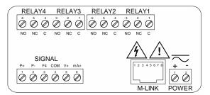
Figure 8. PD6200-##4 Connectors Label
