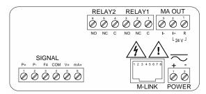
Figure 9. PD6200-##5 Connectors Label
