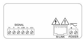
Figure 5. PD6200-##0 Connectors Label
