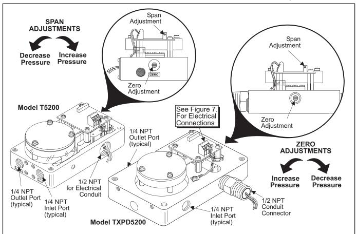
Figure 8. T5200 / TXPD5200 Calibration Configuration.
