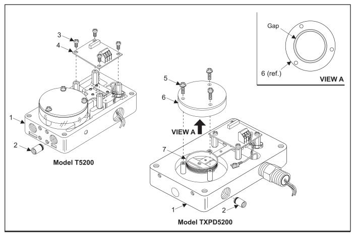
Figure 9. Exploded Drawing.
