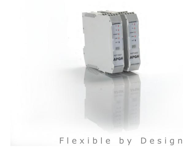
The RST-5000 offers affordable remote tank monitoring by taking your 4-20 mA device and posting the readings to a secure website, sending you an email or a text alarm to your cell phone. Connect up to 10 sensors using the RST-5000 Series as the master for an RS-485 network.
