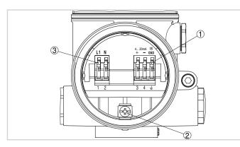
Terminal compartment, double chamber housing
