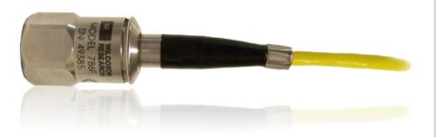
Wilcoxon's top-exit 100 mV/g broadband sensor is ideal for monitoring machine vibration on a wide range of rotating equipment including motors, pumps, fans, compressors, turbines and generators. 316L stainless steel casing provides rugged durability for the most extreme environments. The sensing element is housed in a case-isolated Faraday shield, providing maximum protection from ground loops and RF interference.
