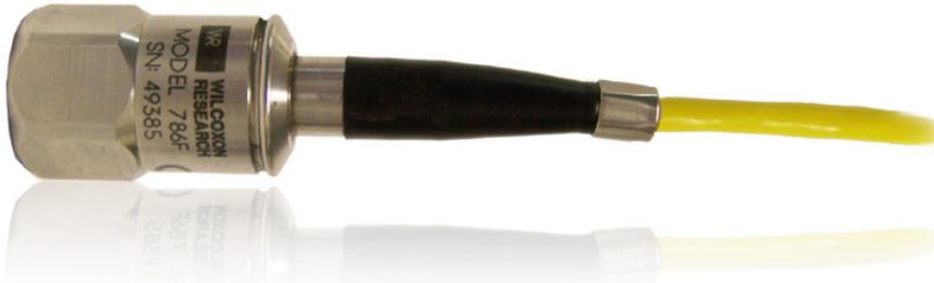
Wilcoxon's top-exit 100 mV/g broadband sensor is ideal for monitoring machine vibration on a wide range of rotating equipment including motors, pumps, fans, compressors, turbines and generators. 316L stainless steel casing provides rugged durability for the most extreme environments. The sensing element is housed in a case-isolated Faraday shield, providing maximum protection from ground loops and RF interference.
