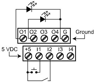
Figure 19. Digital Input and Output Connections
