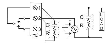
Figure 13. AC and DC Loads Protection
