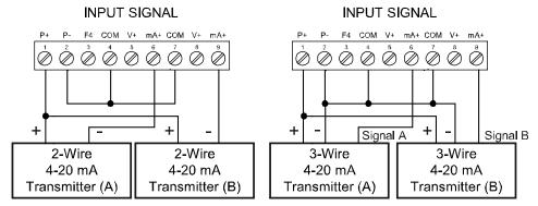
Figure 9. Transmitters Powered by Internal Supply
