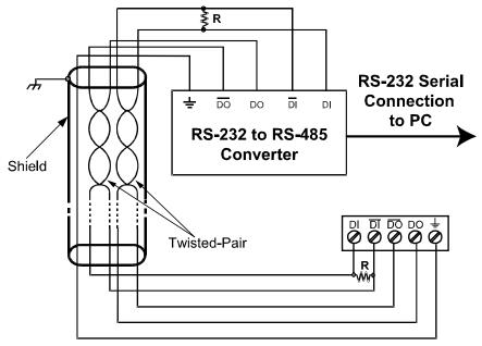
Figure 15. RS-422 or RS-485 Wiring
