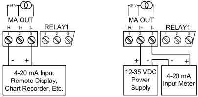
Figure 21. 4-20 mA Output Connections
