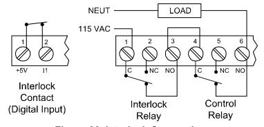
**Figure 22. Interlock Connections**
