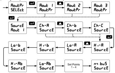
To base an analog output on the rate, total, or grand total of channels A or B, select the channel in the *Analog Output Source* menu. Then select the rate, total, or grand total as the source reference for the output, and program the output scale.
