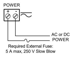
**Figure 8. Power Connections**
