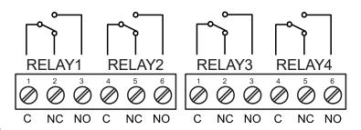
Figure 12. Relay Connections
