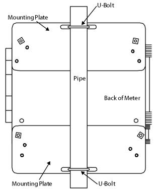
Figure 4. Vertical Pipe Mount Assembly
