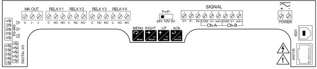
Figure 7. Connector Labeling for Fully Loaded PD2-6262
