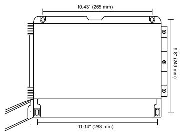
**Figure 1. Meter Mounting Holes**
