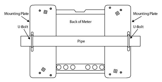
Figure 5. Horizontal Pipe Mount Assembly
