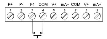
Figure 20. F4 Digital Input Connections
