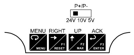
Figure 6. Transmitter Supply Voltage Selection
