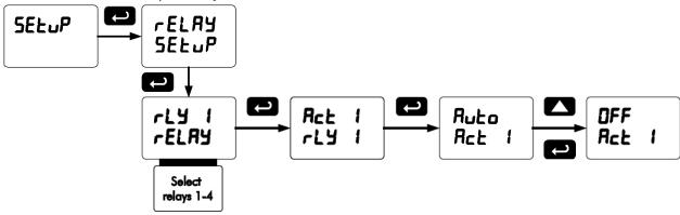
2. In the Advanced features – *User* menu program any of the digital inputs to *Force On* any of the internal relays (1-4).
