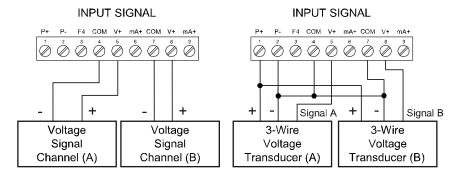
**Figure 11. Voltage Input Connections**
