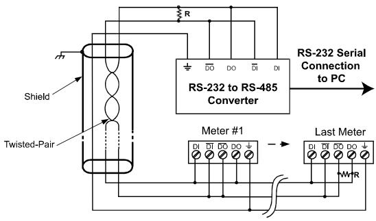
Figure 16. RS-485 Two-Wire Multi-Drop Wiring
