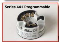
The Series 441 programmable temperature transmitter is a two-wire transmitter with an analog output. It has measurement input for resistance thermometers (RTD) in 2, 3 or 4 wire connection, thermocouples, resistance and voltage. Setting up of the transmitter is done using the 440-CABLE. These small units can be mounted in Pyromation DIN (Form B) heads or they can be used for surface mounting by using a 35 mm DIN rail mounting clip.
