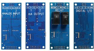
▲ Above: Available base station modules include dual analog input module, dual analog output module, relay module, and Digital I/O module.
