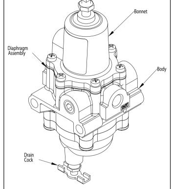
Figure 2. Model 65 Exploded Drawing
