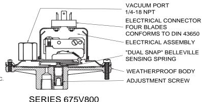
**FIELD SETTING:** Insert 3/16" Allen wrench into adjustment screw (located in pressure port). Clockwise to decrease settings. Counterclockwise to increase settings.
