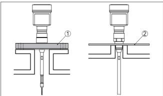
Fig. 3: Mounting in non-metallic vessel
