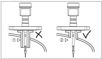
Fig. 5: Socket must be installed flush
