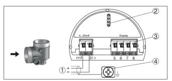
Fig. 8: Connection compartment - double chamber housing
