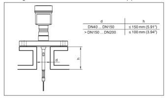
Fig. 4: Mounting socket
