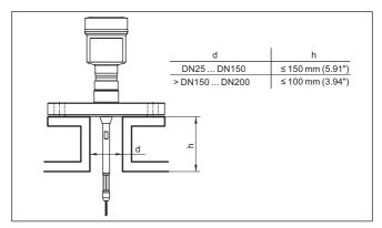
Fig. 4: Mounting socket
