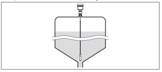
Fig. 2: Vessel with conical bottom
