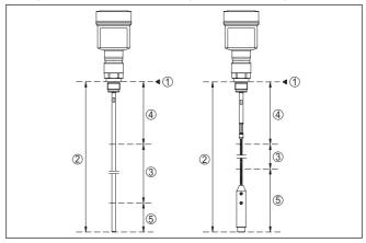
Fig. 11: Measuring ranges - NivoGuide 8100
