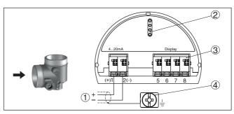
Fig. 8: Connection compartment - double chamber housing
