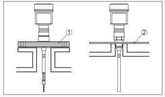
Fig. 3: Mounting in non-metallic vessel
