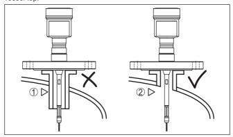
Fig. 5: Socket must be installed flush
