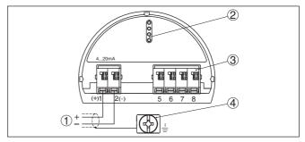
Fig. 7: Electronics and connection compartment - single chamber housing
