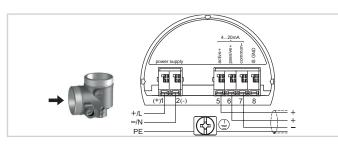
Connection compartment with double chamber housing - mains voltage
