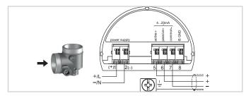
Connection compartment with double chamber housing - low voltage You can find details on electrical connection in the instrument operating instructions at <u>www.vega.com/downloads</u>.
