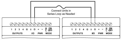
Figure 5. Cascade Mode Multiple Unit I/O Connections
