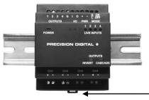
Insert a small slotted screwdriver or similar tool into the mounting tab, and gently pull down on it.
