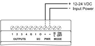
**Figure 2. Power Connections**
