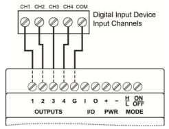
Figure 4. Digital Output Connections
