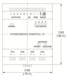
Figure 8. Dimensions - Front View
