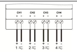
Figure 3. High Voltage Input Channel Connections
