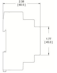
Figure 9. Dimensions - Side View
