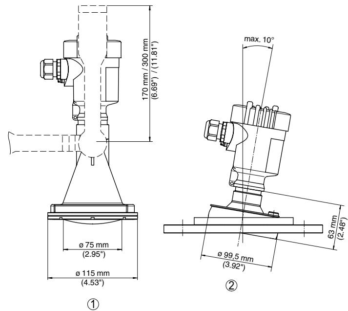
① Plastic horn antenna with mounting strap
