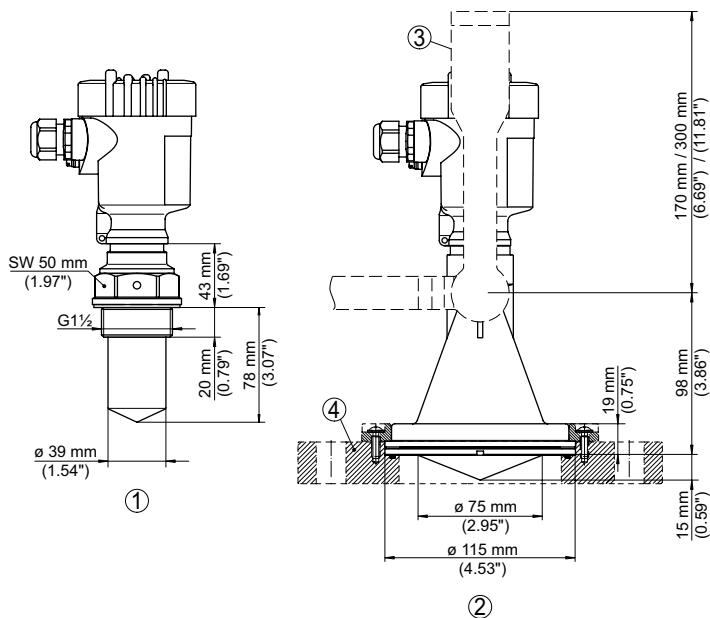
① Version with encapsulated antenna system (Ø 40 mm)
