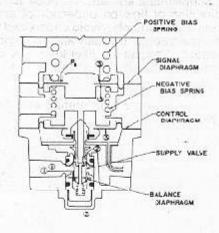
and the range spring force acting on the piston, assisted by the negative bias spring force. This force, acting through the pintle, allows the supply valve to throttle, maintaining the output pressure.
