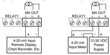
Figure 16. 4-20 mA Output Connections
