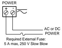
**Figure 4. Power Connections**
