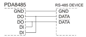
Figure 21: General Two-Wire Network Connection
