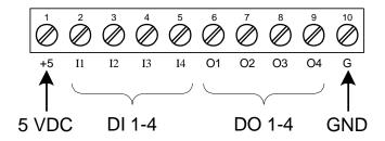
Figure 18: Digital I/O Connections
