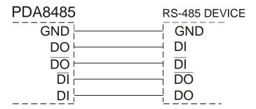
Figure 20: General Four-Wire Network Connection
