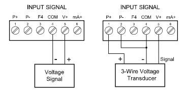
Figure 7. Voltage Input Connections
