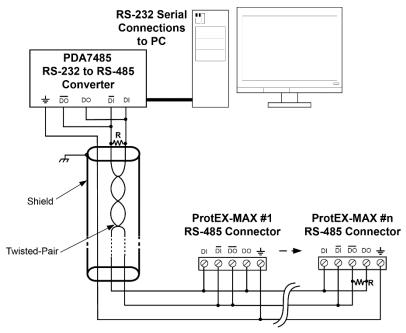
Figure 11: RS-485 Two-Wire Multi-Drop Wiring
