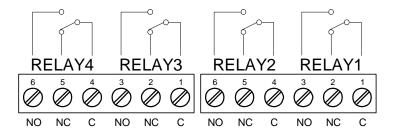
Figure 12. Relay Connections
