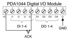
Figure 19. Acknowledge Relays w/ SafeTouch Button or Digital Input Pump Alternation Control Applications (RLEECA)
