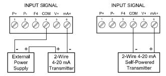
Figure 6. Transmitter Powered by Ext. Supply or Self-Powered
