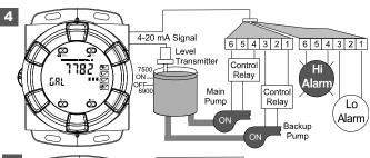
5. Relay #1 trips the Low Level Alarm at 495 gallons and resets at 750 gallons.
