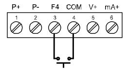
Figure 15. F4 Digital Input Connections
