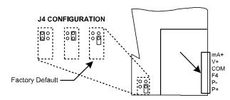
Figure 1. Transmitter Supply Voltage Selection
