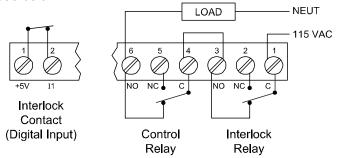
Figure 17. Interlock Connections
