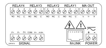
Figure 3. Connector Labeling for Fully Loaded PD6000
