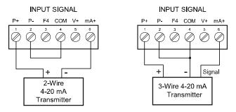
Figure 5. Transmitters Powered by Internal Supply
