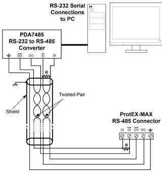
Figure 10: RS-485 Wiring
