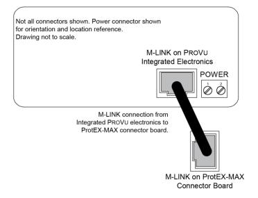
Figure 2: Integrated PROVU Required Connections
