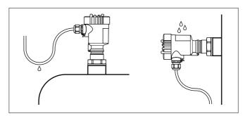
Fig. 2: Measures against moisture penetration
