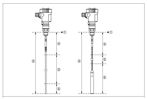
Fig. 27: Measuring ranges of VEGAFLEX 61
