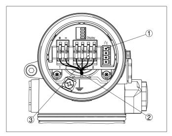
Fig. 13: Electronics compartment, double chamber housing
