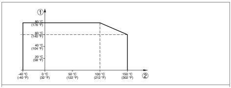
Fig. 34: Ambient temperature - Process temperature
