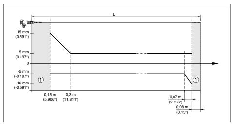
Fig. 29: Deviation VEGAFLEX 61 in rod version in oil
