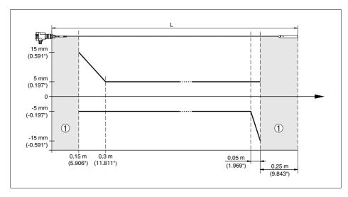
Fig. 31: Deviation VEGAFLEX 61 in cable version, probe length L < 20 m in oil
