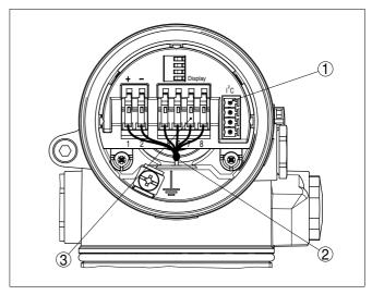
Fig. 16: Electronics compartment, double chamber housing
