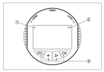
Fig. 21: Indicating and adjustment elements
