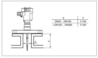
Fig. 6: Mounting socket
