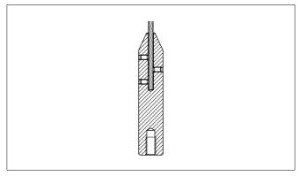
Fig. 26: Shortening the cable probe
