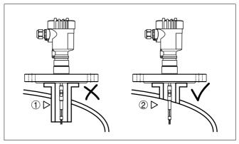
Fig. 7: Socket must be installed flush
