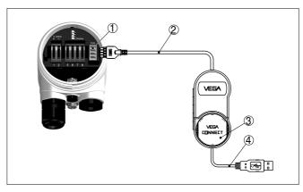
Fig. 23: Connection via VEGACONNECT externally
