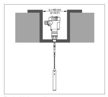
Fig. 5: Installation in concrete silo
