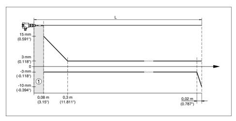
Fig. 28: Deviation VEGAFLEX 61 in rod version in water
