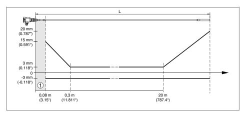
Fig. 32: Deviation VEGAFLEX 61 in cable version, probe length L > 20 m in water
