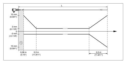
Fig. 30: Deviation VEGAFLEX 61 in cable version, probe length L < 20 m in water
