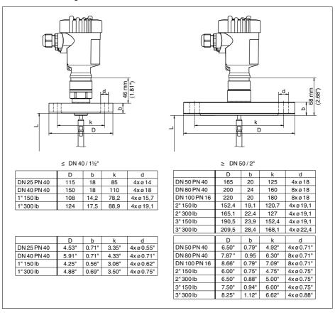
Fig. 41: VEGAFLEX 61 - flange version
