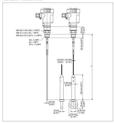
Fig. 40: VEGAFLEX 61 - threaded version
