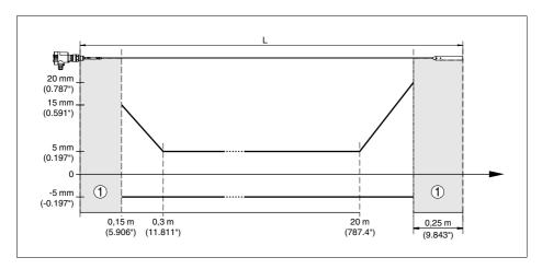
Fig. 33: Deviation VEGAFLEX 61 in cable version, probe length L > 20 m in oil
