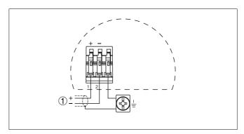
Fig. 18: Wiring plan with double chamber housing Ex d
