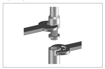
Fig. 25: Exchanging the cable or rod
