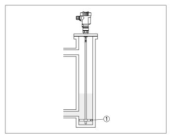
Fig. 8: Position of the spacer
