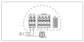
Fig. 12: Wiring plan, single chamber housing
