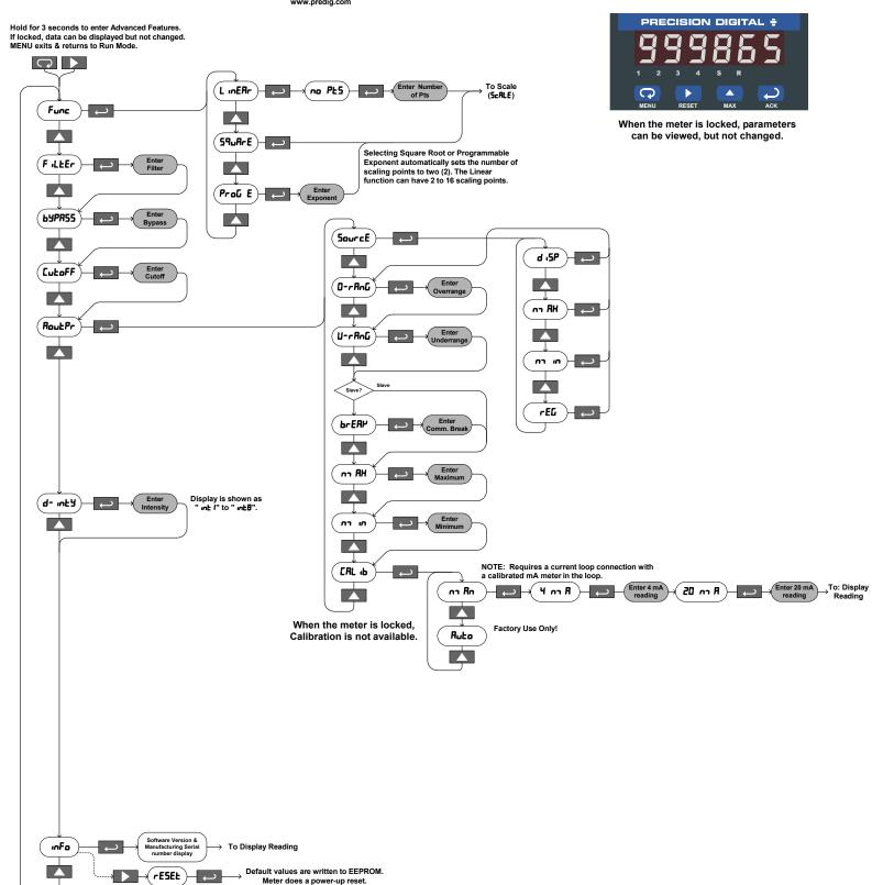
Press and hold for 5 seconds. To Display Reading 3 second timeout. To Display Reading MOTE: Press and hold RIGHT ARROW for 5 seconds while inFo is displayed to enter Meter Reset Defaults mode (display shows rset.) This is used to initialize the EEPROM to factory defaults. Press ENTER to accept. Press MENU or no keys for 3 seconds to exit.
