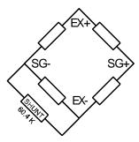
Figure 19. Shunt Resistor
