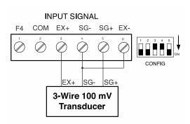
Figure 17. mV Transducer Input Connections
