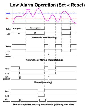
For Manual reset mode, ACK can be pressed anytime to turn "off" relay. For relay to turn back "on", signal must go above set point and then go below it.
