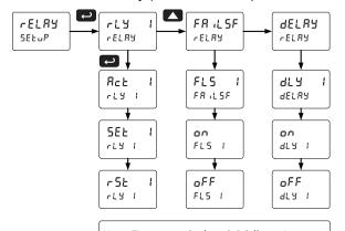
Note: The setup of relays 2-8 follows the same pattern shown here for relay 1.
