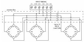
Figure 16. Multiple Strain Gauges Connected
