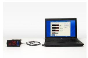
The meter can be powered from the Micro USB connection. When using the Micro USB connection, **DO NOT** apply AC or DC power to the meter.
