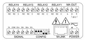
Figure 11. PD6100-##7 Connectors Label
