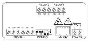
Figure 7. PD6100-##2 Connectors Label
