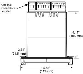
Figure 4. Meter Dimensions - Top View
