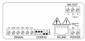
Figure 8. PD6100-##3 Connectors Label
