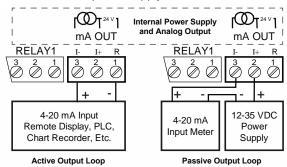
Figure 23. 4-20 mA Output Connections
