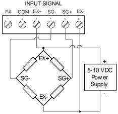
Figure 15. Strain Gauge Powered by External Supply
