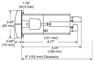
Figure 3. Meter Dimensions - Side View
