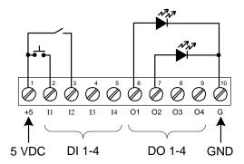
Figure 28. Digital I/O Module Connections
