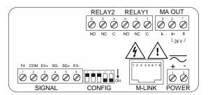
Figure 10. PD6100-##5 Connectors Label
