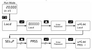
If the correct six-digit password is entered, the meter displays the message unloc (unlocked) and the protection is disabled until a new password is programmed.
