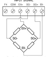
Figure 14. Strain Gauge Powered by Internal Supply
