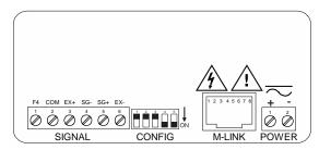
Figure 6. PD6100-##0 Connectors Label
