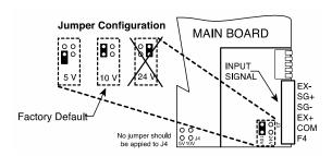
Figure 5. Sensor Excitation Voltage Selection
