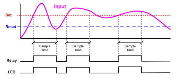
When the signal crosses the set point, the relay trips and the sample time starts. After the sample time has elapsed, the relay resets. The cycle repeats every time the set point is crossed, going up for high alarms and going down for low alarms.
