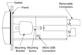
**<u>DO NOT</u>** apply AC or DC power to the meter when using the Micro USB connection.
