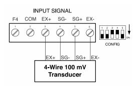
Figure 18. Four-wire mV Transducer Connections
