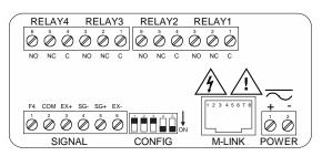
Figure 9. PD6100-##4 Connectors Label
