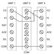
Figure 17. System with Multiple Units Share First-Out
