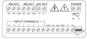
Figure 6. Connector Labeling for PD158-6R2-1
