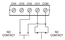
Figure 10. NO/NC Contact Inputs
