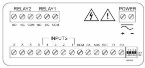
Figure 7. Connector Labeling for PD154-7R2-0
