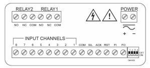
Figure 8. Connector Labeling for PD158-7R2-0
