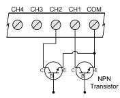
Figure 11. Open Collector NPN Transistor Inputs
