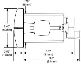
Figure 4. Case Dimensions - Top View
