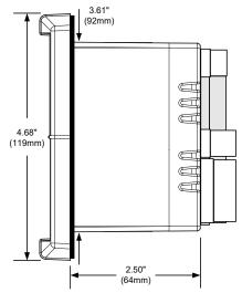
Figure 3. Case Dimensions - Side View
