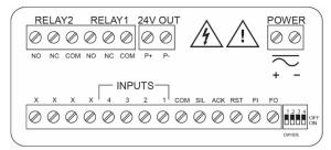
Figure 5. Connector Labeling for PD154-6R2-1
