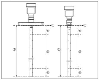
Fig. 8: Measuring ranges - NivoGuide 8100
