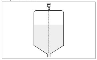
Fig. 2: Vessel with conical bottom
