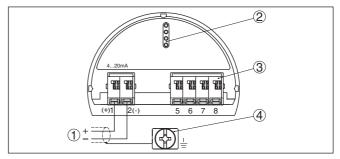
Fig. 4: Electronics and connection compartment - single chamber housing
