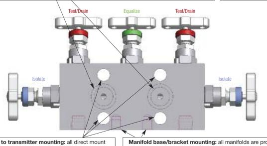
**Manifold to transmitter mounting:** all direct mount manifolds are provided with 4 off 7/16 UNF x 1.625" high tensile zinc plated carbon steel bolts. Bolt holes are standard on 54mm/2.125" centres. Optional St. St. bolts are available.
