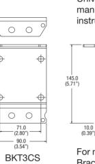
Universal manifold mounting bracket suitable for direct mount manifolds. This bracket design enables horizontal or vertical instrument positioning. Suitable for 2" standpipe.
