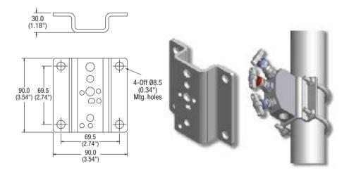
For manifold/bracket bolts add bolt set suffix from matrix. Example: Bracket, 'U' bolt and manifold/bracket bolts BKT2CSB2 (suitable for HL\*3DBB).
