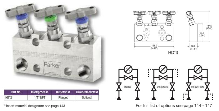
Specifically designed for installation inside enclosures enabling bottom entry connections to be completed outside of the enclosure. Suitable for direct mounting to differential pressure transmitters with 54mm/2.125" mounting centres, supplied with instrument mounting bolts and PTFE seals. Additional test or purge port options are available.
