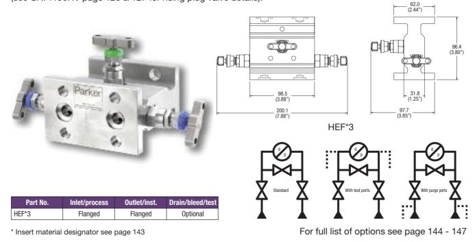
Compact cast body design with optimum positioning of equalize valve for easy access and operation. Manifold suitable for direct mounting to differential pressure transmitters with 54mm/2.125" mounting centres, supplied with instrument mounting bolts and PTFE seals. Additional test or purge port options are available.
