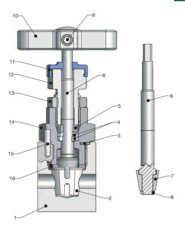
**Standard product specification:** supplied in 316 stainless steel with PEEK soft seat, PTFE packed, T bar operation, 10,000 psig (689 barg) maximum pressure rating, 200C maximum temperature rating.
