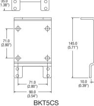
Simple to install bracket on horizontal or vertical 2" standpipe. Designed for horizontal or vertical mounting of manifold giving total installation flexibility.
