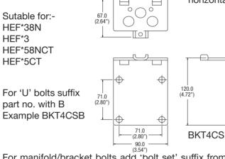
For extruded style manifold blocks providing full base support for horizontal or vertical fixing to 2" standpipe.
