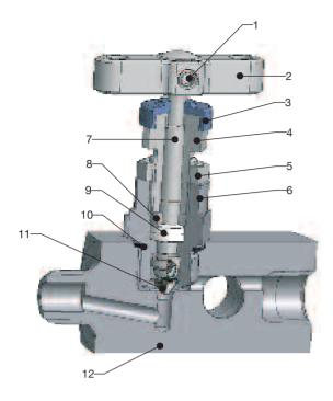
**Standard product specification:** metal/metal seated, PTFE packed, stainless steel, T bar operation, globe pattern, 1/4" NPT vent/bleed port, 6,000 psig (414 barg).
