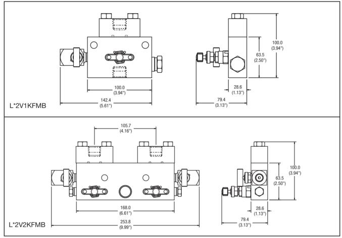
Overall width with valves fully open
