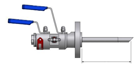
The probe length must be specified from the raised face to the end of the probe in mm, to the nearest mm. Probes are supplied to suit the insertion length required by the pipeline and thus must be specified by the customer. A wide variety of end preparations and support collars are available on request.
