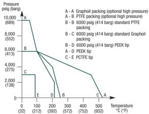
**Standard product specification:** metal/metal seated, PTFE packed, stainless steel, T bar operation, globe pattern, 6000 psig (414 barg).
