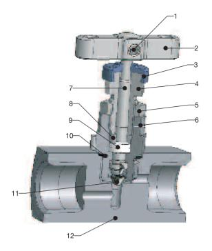
**Standard product specification:** metal/metal seated, PTFE packed, stainless steel, T bar operation, globe pattern, 6000 psig (414 barg).
