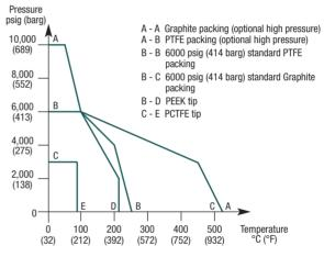
**Standard product specification:** metal/metal seated, Graphite packed, stainless steel, T bar operation, inline pattern, 6000 psig (414 barg).
