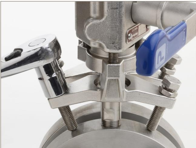
Using a torque wrench tighten the 2 flange mounting bolts (19mm (3/4") A/F Hex) to 33 N.M (300 lb.in). At this stage ensure the lock nuts do not contact the foot
