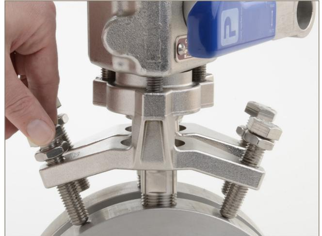
Hand tighten the flange mounting bolts onto the flange. At this stage ensure the lock nuts do not contact the foot
