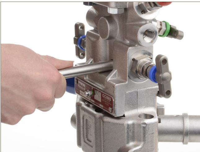
Press down on the handle. The two modules are fully engaged when green safety indicator is deployed
