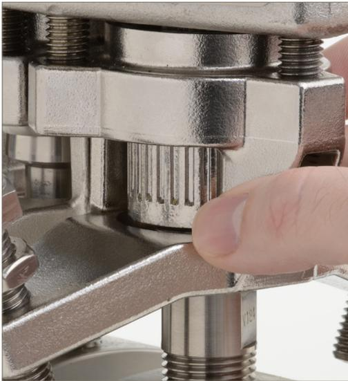
Engage the splined nut onto the thread by 1 - 2 rotations.
