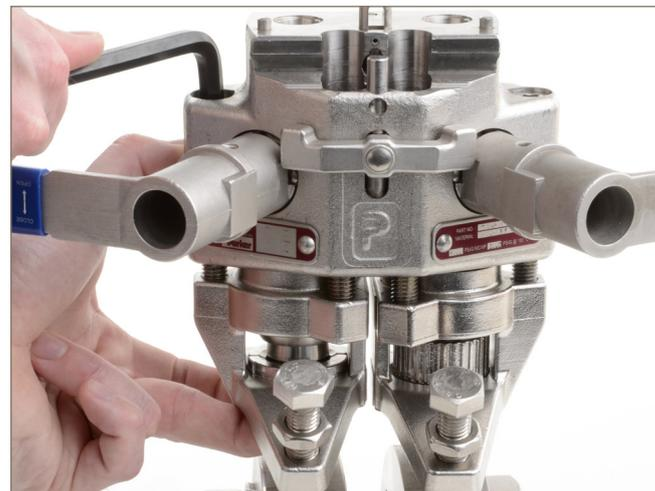
Holding the foot in position, tighten the swivel side retaining bolts (8mm socket cap head x 3) until finger tight i.e. zero torque / effort
