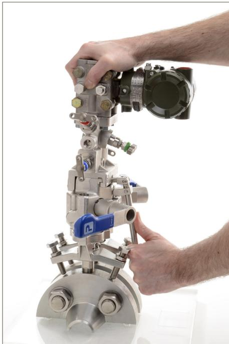
Holding the secondary module, depress the assembly tool handle to unlock the modules
