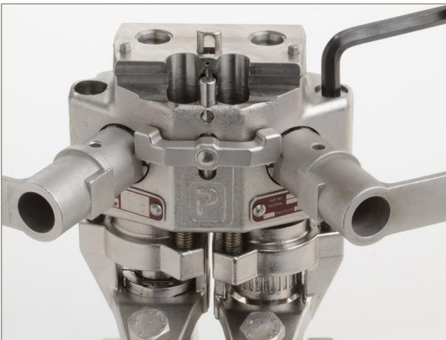
Tighten the slide side retaining bolts (8mm socket cap head x 3) until finger tight i.e. zero torque/effort
