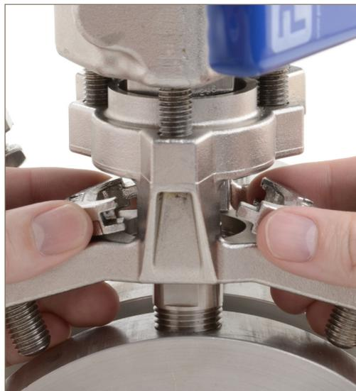
Align and engage the split rings around the swivel tapping collar (as shown)
