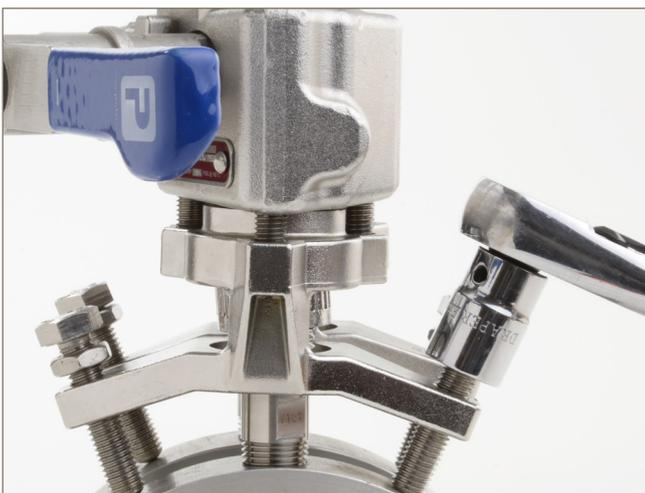
Using a torque wrench tighten the 2 flange mounting bolts (19mm (3/4") A/F Hex) to 33 N.M (300 lb.in). At this stage ensure the lock nuts do not contact the foot
