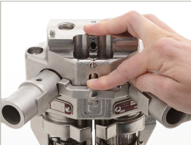
To re-engage the interlock, press and hold both the interlock bar and plunger
