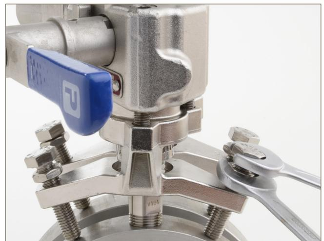
Using 2 spanners tighten to lock nut (19mm (3/4") A/F Hex)
