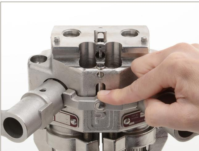
Release the interlock plunger while holding the bar. The interlock bar will latch into the engaged position
