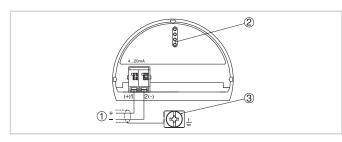
Electronics and terminal compartment, single chamber housing
