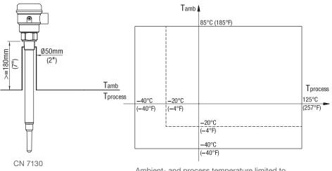
Ambient- and process temperature limited to -20°C (-4°F) with option FFKM seal O-ring
