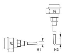
\* Switchpoint is below the probe (material not touching the probe).
