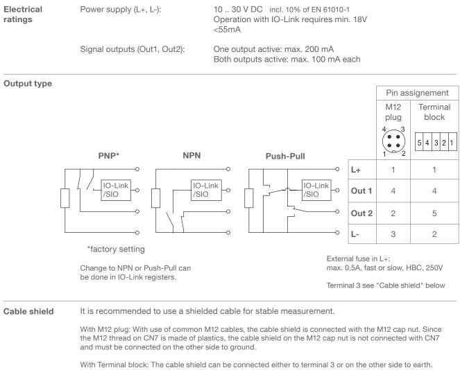
With Terminal block: The cable shield can be connected either to terminal 3 or on the other side to earth. Do not connect both sides of the shield to earth. Note: terminal 3 is internal connected to the external equipotential bonding terminal on the enclosure.
