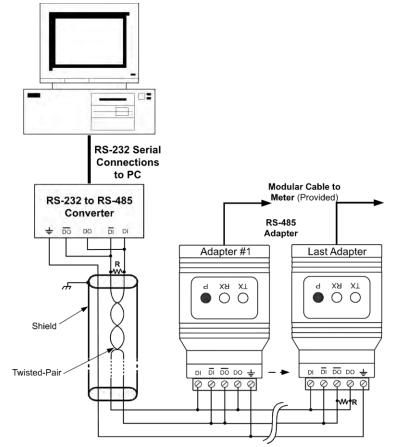
Figure 10. RS-485 Two-Wire Multi-Drop Wiring
