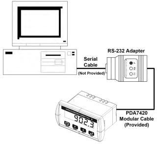
Figure 7. RS-232 Adapter Connections
