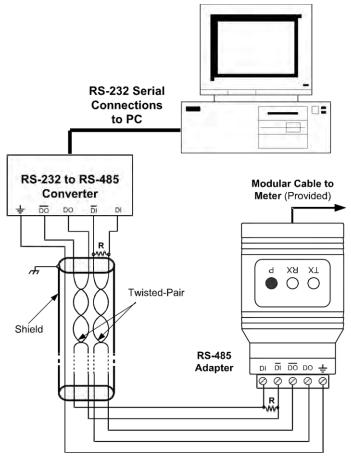
Figure 9. RS-422 or RS-485 Wiring
