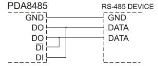
Figure 2. General Two-Wire Network Connection
