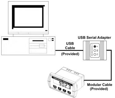
Figure 18. USB Adapter Connections
