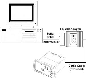
Figure 3. RS-232 Adapter Connections
