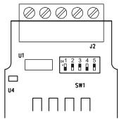
Figure 24. PDA8485 DIP Switch Location
