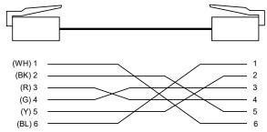
Figure 11. Standard Modular Cable Wiring
