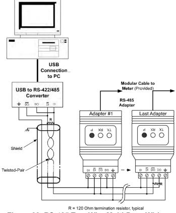
Figure 28. RS-485 Two-Wire Multi-Drop Wiring
