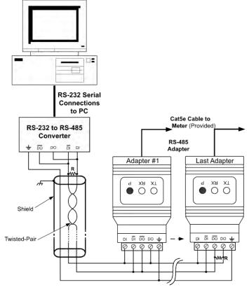
Figure 5. RS-485 Two-Wire Multi-Drop Wiring
