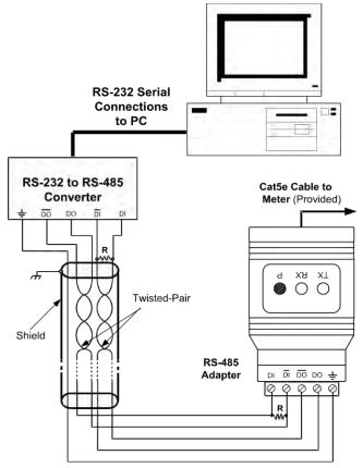
Figure 4. RS-422 or RS-485 Wiring
