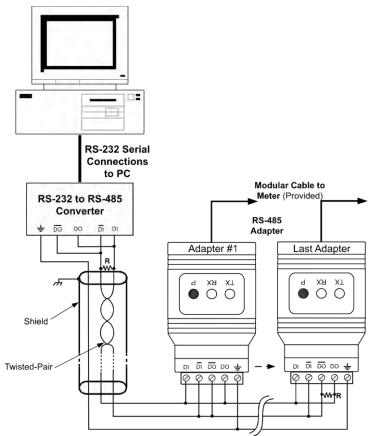
Figure 15. RS-485 Two-Wire Multi-Drop Wiring
