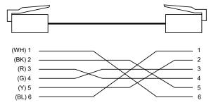
Figure 8. Standard Modular Cable Wiring
