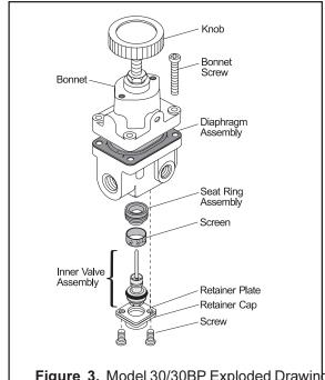
Figure 3. Model 30/30BP Exploded Drawing
