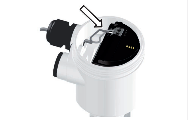
Fig. 16: Connection steps 5 and 6 - Single chamber housing
