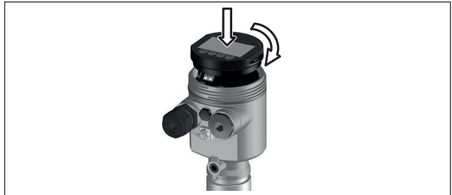
Fig. 23: Installing the display and adjustment module in the electronics compartment of the single chamber housing
