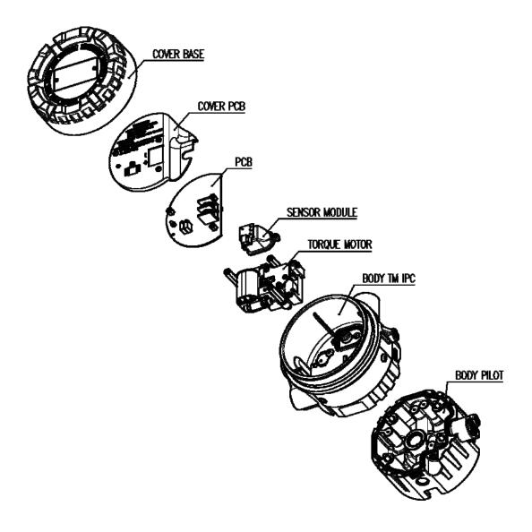
As input signal is being supplied to YT-940, the pressure sensor which is being connected to output port, will sense the pressure level. The main PCB will compare the input signal and output pressure level and increase or decrease the electric current of torque motor.
