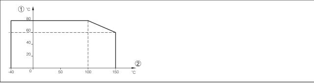
Fig. 17: VEGAFLEX 63 - ambient temperature - product temperature
