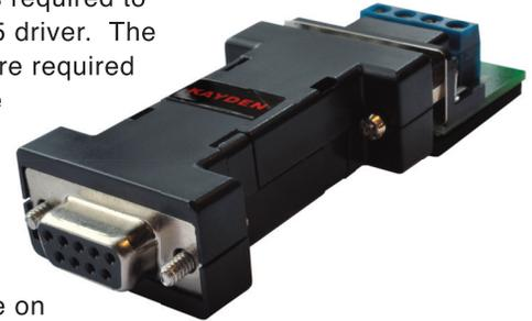
The SCA-321 has an internal connection to prevent data transmitted from the RS-232 port from being echoed back to the RS-232 port. The SCA-321 is used as a two-wire (half duplex) RS-485 converter with a third conductor to be used as signal ground. Using a common signal ground ensures that the common mode voltage between devices falls within the specifications of RS-485. This is especially important for networked devices with opto-isolated RS-485 interfaces.
