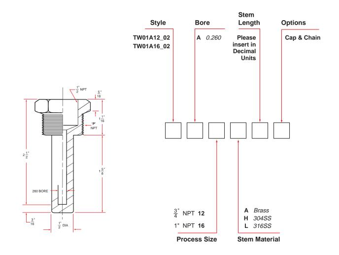
Application: used where a short insertion length is necessary as in short legs of tees etc. This "well" also fits the 2  $1/_2$ " length. Bi-metal thermometer with  $1/_4$ " stem diameter.
