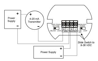
Figure 6. Connections with Externally-Powered Backlight
