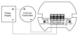
Figure 4. Connections without Backlight
