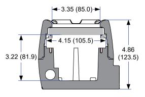
Figure 2. Enclosure Dimensions – Side Cross Section View
