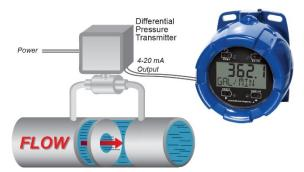
PD6800 Displaying Flow Rate by Extracting Square Root from DP Transmitter Signal.
