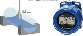
PD6800 Displaying Volume in Round Horizontal Tank Using Multi-Point Linearization Feature
