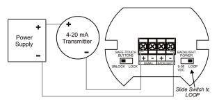
Figure 5. Connections with Loop-Powered Backlight
