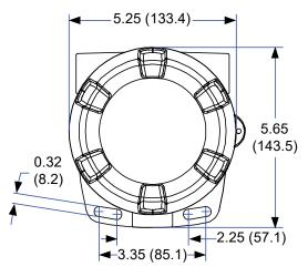
Figure 1. Enclosure Dimensions – Front View
