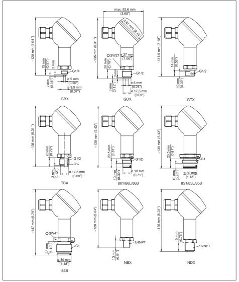
Fig. 20: VEGABAR 17 terminal housing, GBX =  $G^{1/2}$  B manometer connection, GDX =  $G^{1/2}$  B manometer connection, GTX =  $G^{1/2}$  A according to DIN 3852-E, TBX =  $G^{1/2}$  B, inside  $G^{1/4}$  B, 84B = G1 B front-flush max. 25 bar, 851/85L/85B = G1 B front-flush with O-ring up to 1.6 bar, 861/86L/86B =  $G^{1/2}$  B front-flush with O-ring > 1.6 bar, NBX =  $\frac{1}{4}$  NPT thread, NDX =  $\frac{1}{2}$  NPT thread
