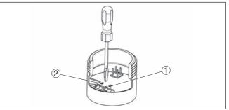
Fig. 16: Adjustment of zero and span
