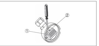
Fig. 14: Adjustment of zero and span
