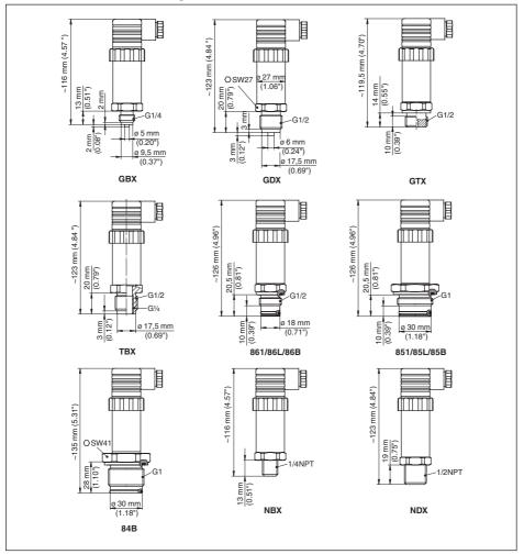
Fig. 18: VEGABAR 17 standard housing, GBX = G½ B manometer connection, GDX = G½ B manometer connection, GTX = G½ A according to DIN 3852-E, TBX = G½ B, inside G¼ B, 84B = G1 B front-flush max. 25 bar, 851/85L/85B = G1 B front-flush with O-ring up to 1.6 bar, 861/86L/86B = G½ B front-flush with O-ring > 1.6 bar, NBX =  $\frac{1}{2}$  NPT thread, NDX =  $\frac{1}{2}$  NPT thread
