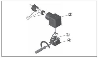
Fig. 7: Connection to the screw terminals
