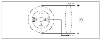
Fig. 10: Wiring plan, angle plug connector according to ISO 4400, top view to VEGABAR 17
