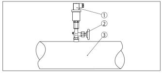
Fig. 3: Measurement setup for process pressure measurement of gases in pipelines
