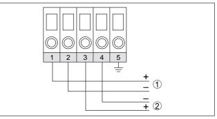
Fig. 13: Wiring plan, terminal housing
