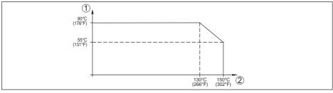
Fig. 17: Temperature derating VEGABAR 17
