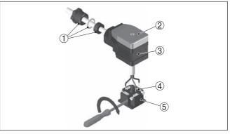
Fig. 9: Connection to the screw terminals
