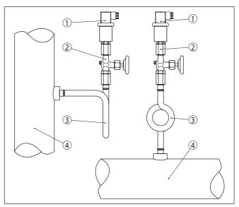
Fig. 4: Measurement setup for the process pressure measurement of gases in pipelines
