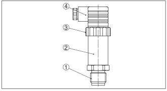
Fig. 1: VEGABAR 17 with plug connector according to ISO 4400
