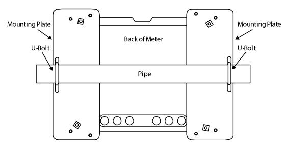
Figure 5. Horizontal Pipe Mount Assembly
