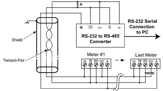
Figure 16. RS-485 Two-Wire Multi-Drop Wiring
