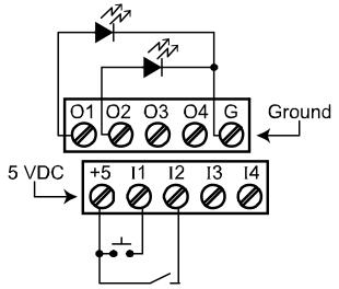
Figure 19. Digital Input and Output Connections
