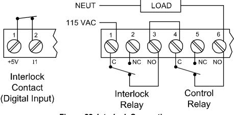
Figure 22. Interlock Connections
