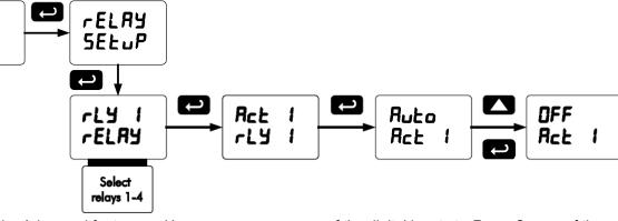
2. In the Advanced features – *User* menu program any of the digital inputs to *Force On* any of the internal relays (1-4).
