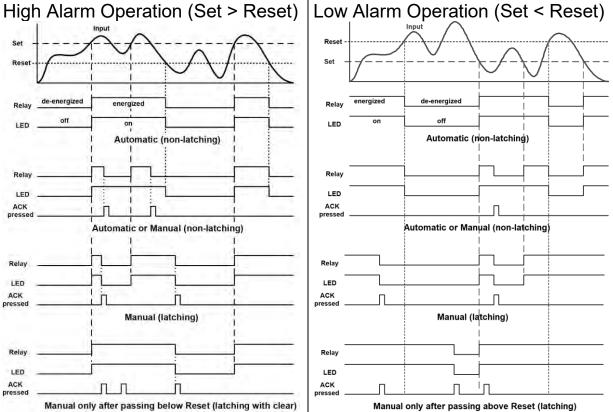
For Manual reset mode, ACK can be pressed anytime to turn "off" relay. To detect a new alarm condition, the signal must go below the set point, and then go above it. For Manual reset mode, ACK can be pressed anytime to turn "off" relay. For relay to turn back "on", signal must go above set point and then go below it.
