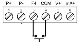
Figure 20. F4 Digital Input Connections
