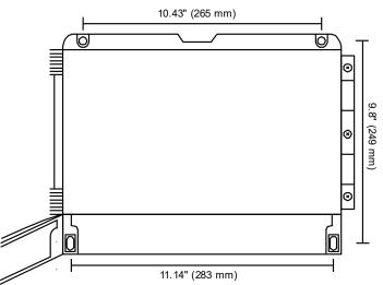
Figure 1. Meter Mounting Holes
