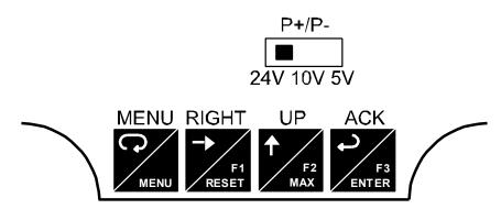
Figure 6. Transmitter Supply Voltage Selection
