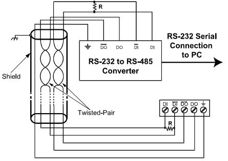
Figure 15. RS-422 or RS-485 Wiring
