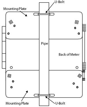
Figure 4. Vertical Pipe Mount Assembly
