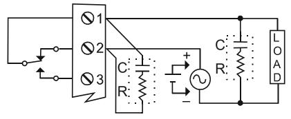
Figure 13. AC and DC Loads Protection
