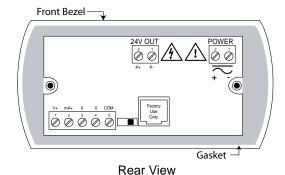
Meter with 24 V Transmitter Supply Option
