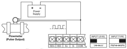
Figure 2. Flowmeter Powered by External Supply
