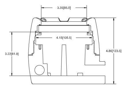
Figure 15. Enclosure Dimensions – Side Cross Section View
