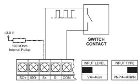
Figure 7. Switch Contact Input
