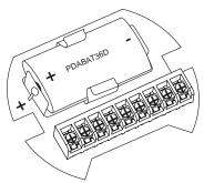
Figure 11. Battery Orientation
