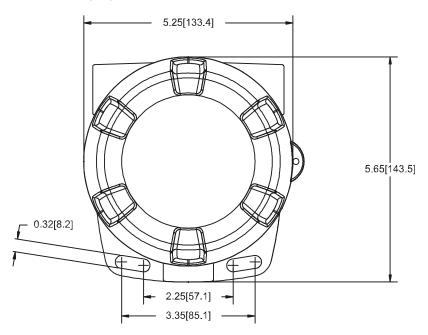
Figure 14. Enclosure Dimensions – Front View
