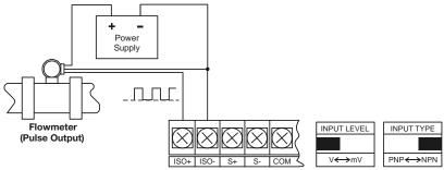
Figure 3. Opto-Isolated Flowmeter Powered by External Supply
