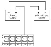
Figure 10. 4-20 mA Output Connections
