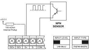
Figure 5. NPN Open Collector Input
