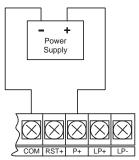
Figure 8. DC Power Connections
