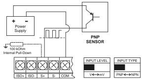
Figure 6. PNP Sensor with External Power
