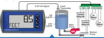
Relay #2 turns the main pump on at 8.5 Feet and turns it off at 3.5 Feet.
