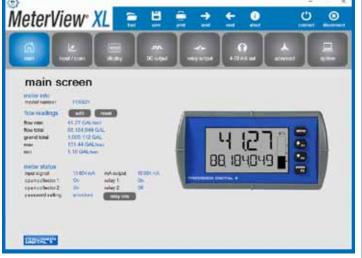
The main screen displays an image of the connected meter and includes various information about this meter, such as model number, readings, and status.
