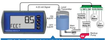
With the Pump Alternation feature activated, the next time the level reaches 8.5 Feet, relay #1 transfers and starts the backup pump.
