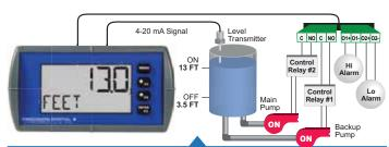
If the backup pump is not able to keep up, and the level reaches 13.0 Feet, relay #2 transfers and starts the main pump as well.
