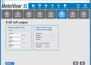
▲ The 4-20 mA Output window is used to program the isolated 4-20 mA output's source, range, and under and over range values.
