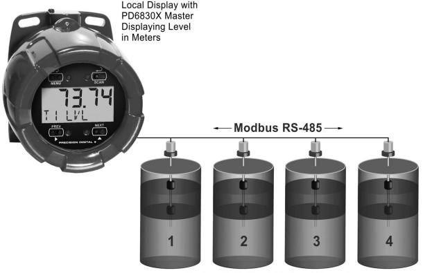
Tanks with Multivariable Level Transmitters
