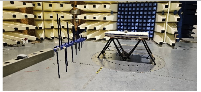
Fig H2 Radiated Emissions 300MHz -1GHz 3metres
