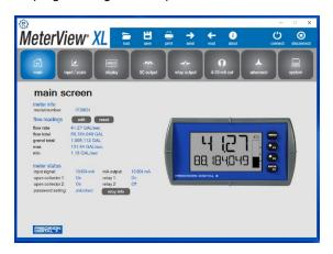
All models come equipped with two open collector outputs and are available with two solid state relays and isolated 4-20 mA analog output options. The open collector outputs are useful for alarm indication or pulse output. The relays can be programmed for alarm indication, on/off control, or pump alternation.
